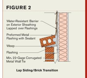
For the vertical joint between these sections, a J-channel and sealant should be enough to close off the gap. Other trim pieces may also be used, as long as they redirect water. A more difficult transition occurs in the horizontal direction when the lap siding is placed above brick veneer. Durable flashing must cover the gap created by the air space behind the brick (see Figure 2).
